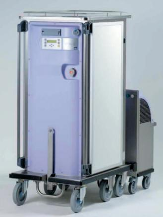
The tray with food from the meal plating belt is placed into the trolley (capacity 16, 20, 24, 28 & 30 level). Once loaded the trolley is docked with a Stand-Fresh compressor unit for a 20 minute boost period whereby the hot shelves are thermalised and the cold section chilled at each level during the same cycle. The trolley is then un-docked and transported to ward level with temperatures
